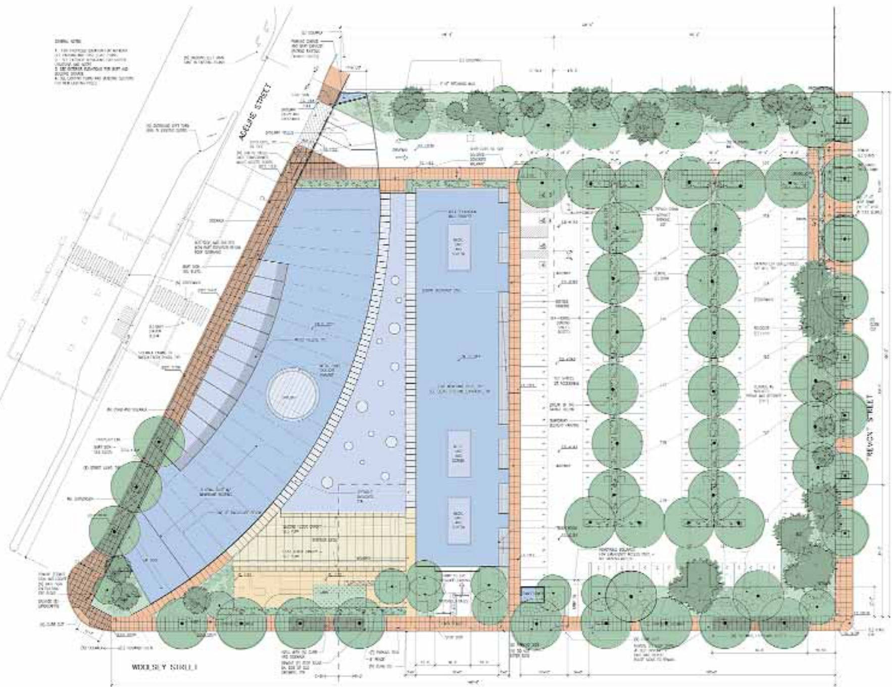
The site plan shows access for BART patron parking via a new driveway at the northwest corner of the site at Adeline Street.
